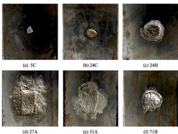
Fig. 1. Photographs of corrosions introduced into six of the samples. The size of the photographs is 5 cm x 5 cm.
