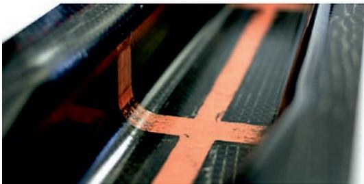
Fig. 12. Hut profile, upper with integrated SHM network.
