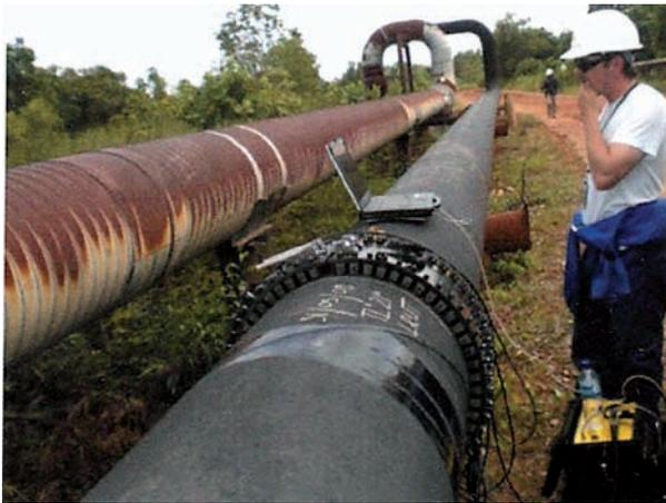
Fig. 3. Low-frequency ultrasonic diagnostics
