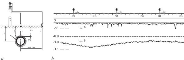
Fig. 1. Evaluation of quality of pipeline insulation based on results of measurement of polarization potential  $U_p$ : a – scheme; b – measurement results,  $U_{mg}$  – potential between pipe and electrode,  $U_{gg}$  – the same at  $x$  distance from axis,  $h$  – pipeline burial depth
