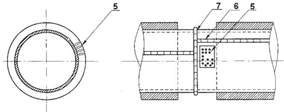
Fig. 9. Position of code panel (5) in zone of intersection of longitudinal (6) and assembly (7) welds
