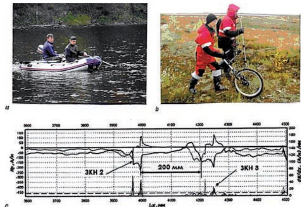
Fig. 2. Magnetometric diagnostics determining stress concentration zones (scz): a, b – measurement process; c – surface distribution  $H$  (A/m) of magnetic field intensity and its gradient  $dH/dx$  along main pipe axis
