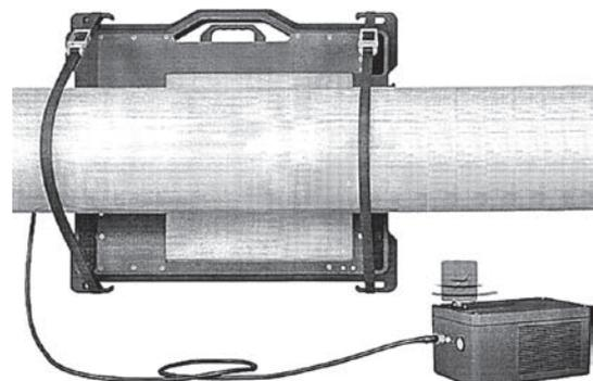
Fig. 6. Pipeline corrosion damage examination with a usage of DRP2020NDT
