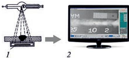
Fig. 3. Quick X-ray inspection scheme without intermediate carriers of information: (1) solid flash-transducer; (2) digital image
