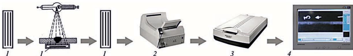
Fig. 1. Traditional scheme of radiographic testing with film and X-ray patterns digitization: (1) cartridge with X-ray film; (2) processing of X-ray film; (3) image scanning; (4) digital image
