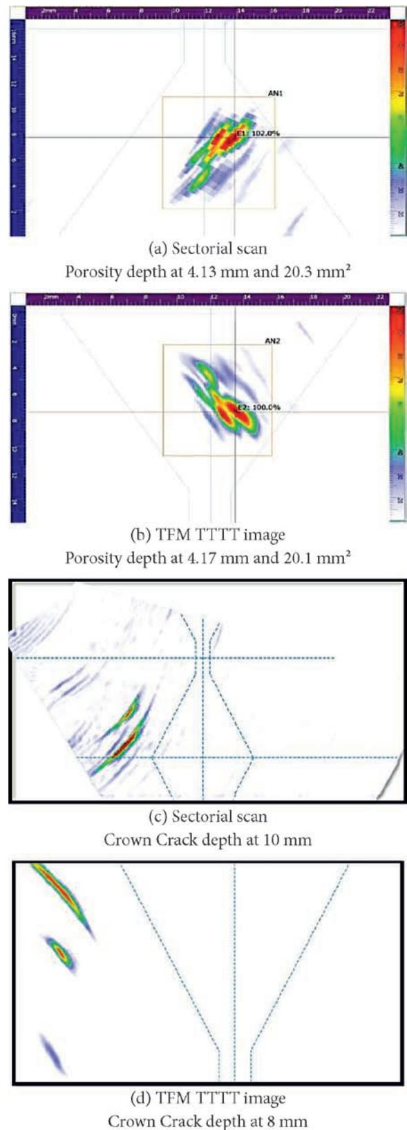
Fig. 8. Sectorial scan (32E) and TFM imaging comparisons.
