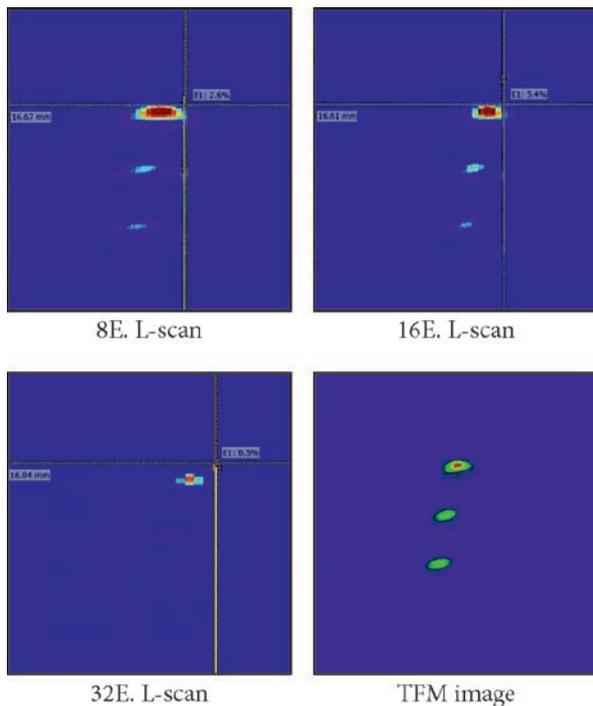
Fig. 4. AWS resolution block with three SDH vertically aligned.
