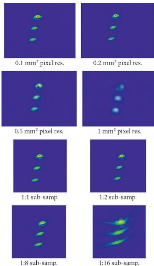
Fig. 6. Pixel resolution and sub-sampling the A-scan comparison.
