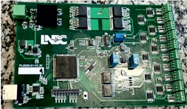
Fig. 7. Photo of the electronic hardware developed to drive and measure the EC transducer impedance variation.
