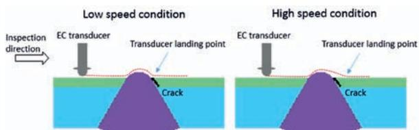
Fig. 2. Influence of the weld geometry and the inspection speed in the crack detectability.
