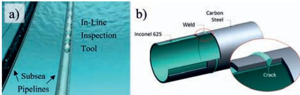
Fig. 1. A) Subsea pipelines and the in-line inspection tool (PIG), and B) Clad pipe section with the inspection region highlighted.
