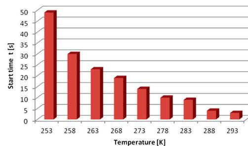
Fig. 3. Effect of temperature on motor starting time
