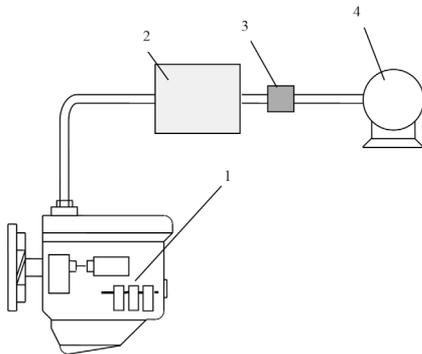
Fig. 1. Schematic of the research station: 1-test engine, 2-expansion tank, 3-gas purification filter, 4-gas meter laboratory.
