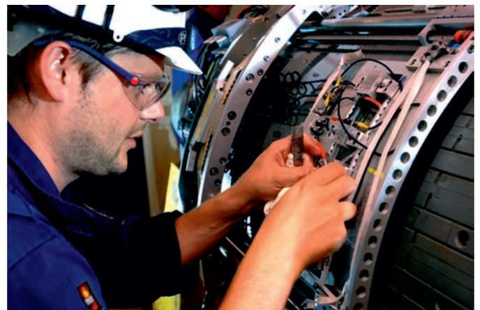
Fig. 3. End Ring Inspection
