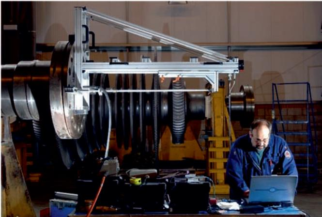
Fig. 1. Rotor Bore Inspection
