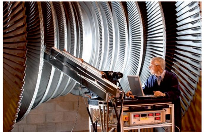
Fig. 2. Rotor Disc Bore Inspection
