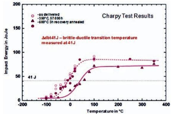
Fig. 3. Charpy Test Results of WB 36
