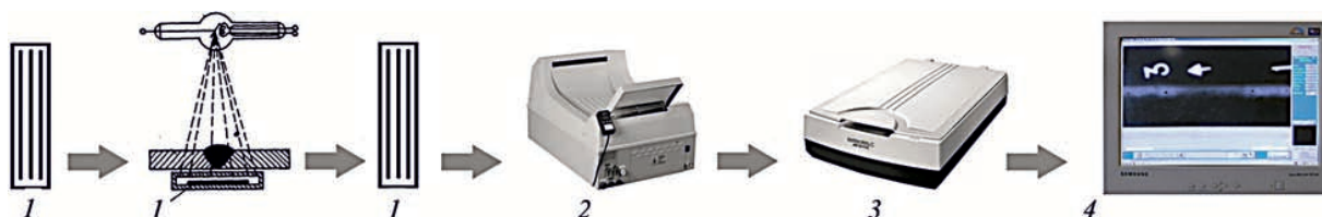
Fig. 1. Traditional scheme of radiographic testing with film and X-ray patterns digitization: (1) cartridge with X-ray film; (2) processing of X-ray film; (3) image scanning; (4) digital image
