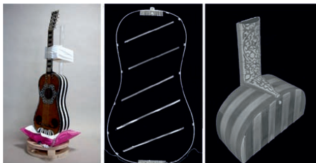
Fig. 6. Investigation of a precious guitar built in the first half of the 17th century in Italy [14]: Photography of the specifically designed support construction of the instrument (left), horizontal slice through the stabilizing structures inside the resonance body of the instrument (center), a surface rendered 3D display of the delicate ornaments embedded into the corpus and the neck (right).
