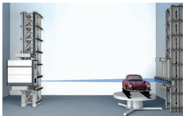
Fig. 8. High Energy CT at Fraunhofer EZRT: Schematic presentation of the set-up of the high-energy facility.
