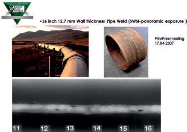
Fig. 1. Inspection of welded pipelines with CR [6]
